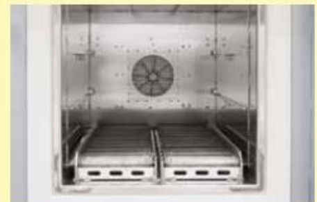
Roller conveyor in furnace chamber
